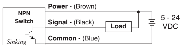
NPN wiring connection - both NC &amp; NO
