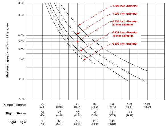
Maximum "D" distance between bearing supports - inches (mm)
