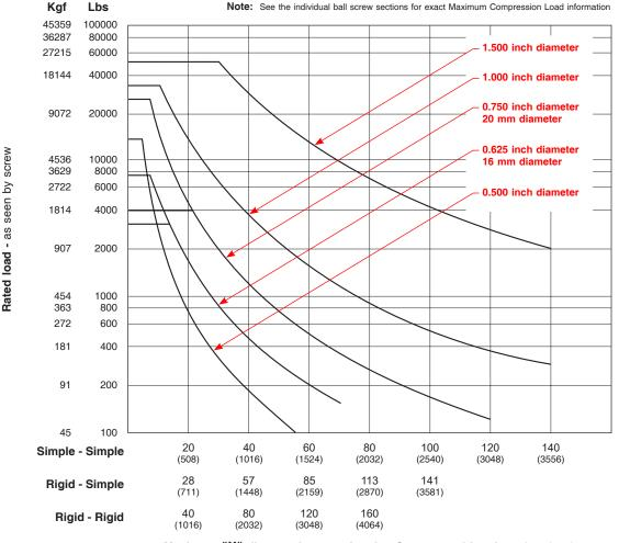
Maximum "X" distance between bearing Support and Load - inches (mm)
