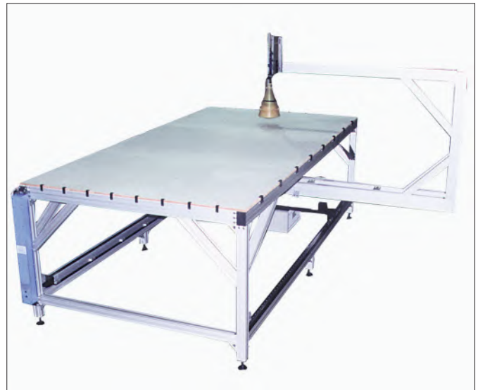
Belt driven long travel X-Y-Z inspection station with aluminum support structure
