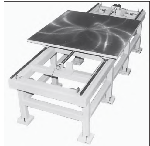
X axis machining station with steel support structure
