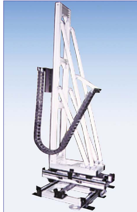
X-Y-Z automated assembly system with aluminum support structure
