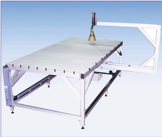
Belt driven long travel X-Y-Z inspection station with aluminum support structure
