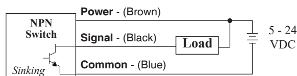
NPN wiring connection - both NC &amp; NO
