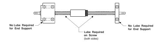
Two *LINTECH* Ball Screw Assembly series come standard with a lube hole in the side of the ball nut. This hole is a 1/8-27 NPT, and the location is shown in the below diagram. This can be used for an automated lubrication tube to disperse oil directly into the nut if required. This is available only with the RS150050, and RS150200 series.
