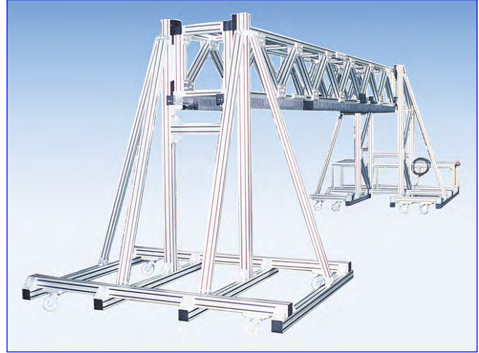
X-Y belt driven infrared inspection station supported by movable aluminum structure
