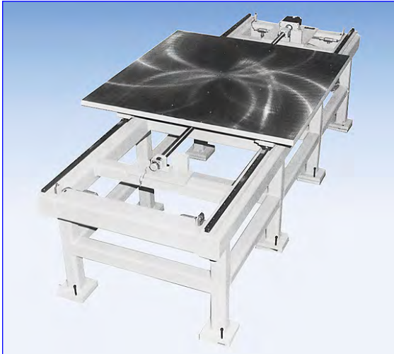
X axis machining station with steel support structure
